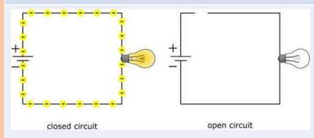
Scientific symbols are used to represent the components (parts) of a circuit in a simple circuit diagram.
